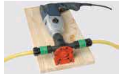
Unser Tipp: Pumpe + Bohrmaschine + Brett
