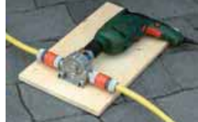
Unser Tipp: Pumpe + Bohrmaschine + Brett
