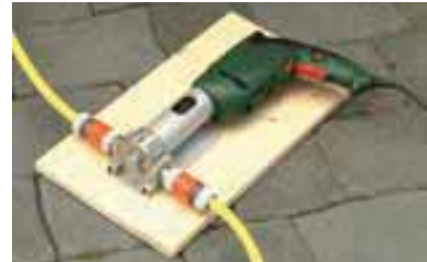
Unser Tipp: Pumpe + Bohrmaschine + Brett
